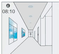
4 When the natural light level exceeds setpoint off to light, the light will turn off even if when the space is occupied.
