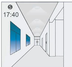
5 The light automatically turns on at 10% when natural light is insufficient (no motion).
