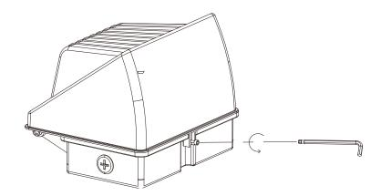
2.Drill 2 holes (0.125 inch) through fixture, and 2 holes into mounting surface using drill template. Drive wall anchors into holes. Attach the fixture to wall with using 2 screws (not included).
