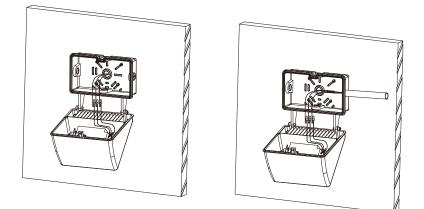
5. Close hatch and tighten M3x12mm locking screw with 3mm allen wrench.
