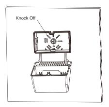
4. Pull wires from conduit through knockout and make wire connections to main supply. Black to Line, White to Neutral, and Green to Ground. Consult an electrician and install according to national, local, and state codes.
